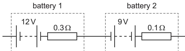
Battery 1 has electromotive force (e.m.f.) 12V and internal resistance 0.3Ω.
