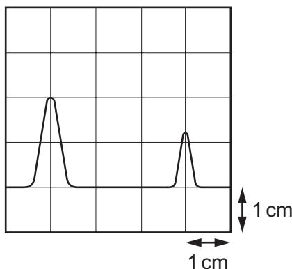
The pulse takes  $6.3 \mu\text{s}$  to travel from the transmitter to the reflector.
