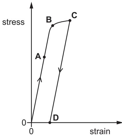
21 A tensile force is applied to an unstretched rubber band, causing it to stretch. The tensile force is then removed.
