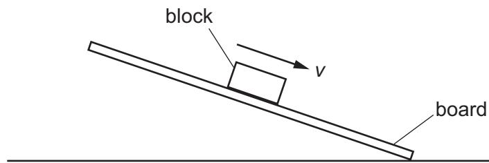
What describes the forces acting on the block when it is sliding with constant velocity?
