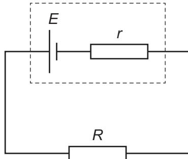
What is the maximum value of  $E$  if the resistor does not overheat?
