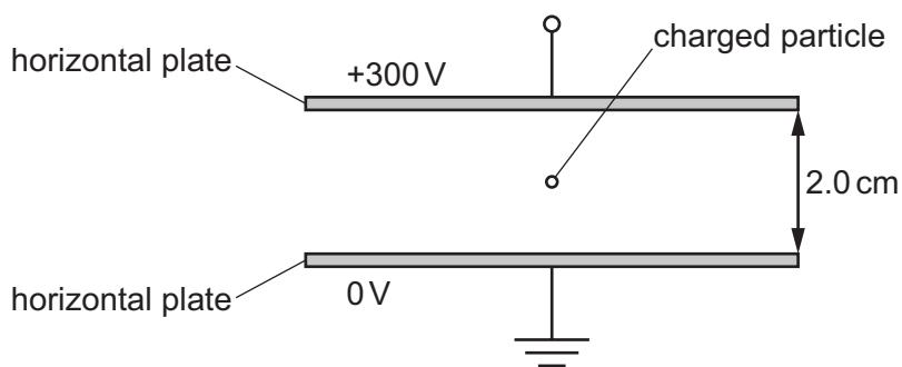
The acceleration of the particle is  $7.15 \times 10^{11} \text{ m s}^{-2}$  downwards. The particle has a mass of  $3.34 \times 10^{-27} \text{ kg}$ .
