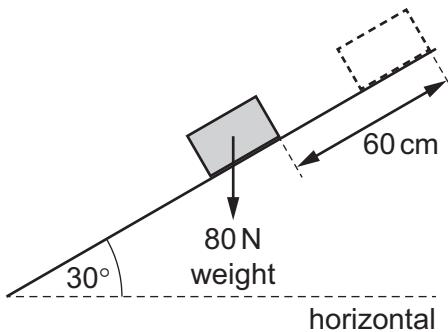
What is the work  $W_g$  done against the gravitational force and the work  $W_f$  done against the frictional force?
