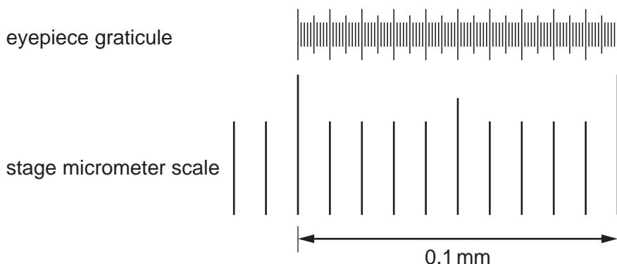
How is the value, in  $\mu\text{m}$ , of one eyepiece graticule unit calculated?
